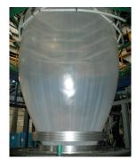
Once it is thoroughly mixed, put the said mixture into the hopper of the extruder for extrusion into film. We recommend that only virgin P.E. resin should be used for production of VCI film. If necessary, modifications are made to provide for any additional properties needed such as UV, Anti-Static, etc...
